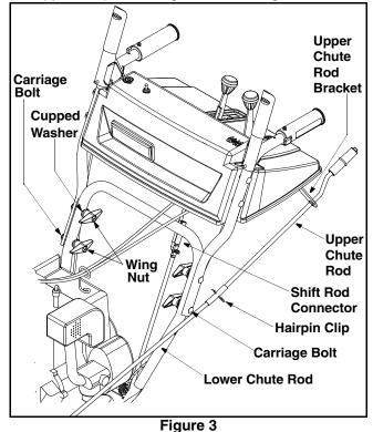
• Slide the shift rod connector down over the end of the lower shift rod. Tap the connector until it **locks** on the lower shift rod. See Figure 3.
